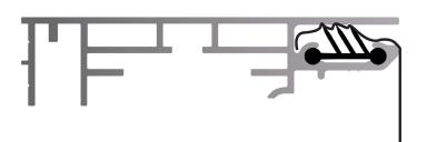
EASITEX has an internal "grip-strip" which clamps the fabric firmly into position leaving you with a great and hassle-free finish.
